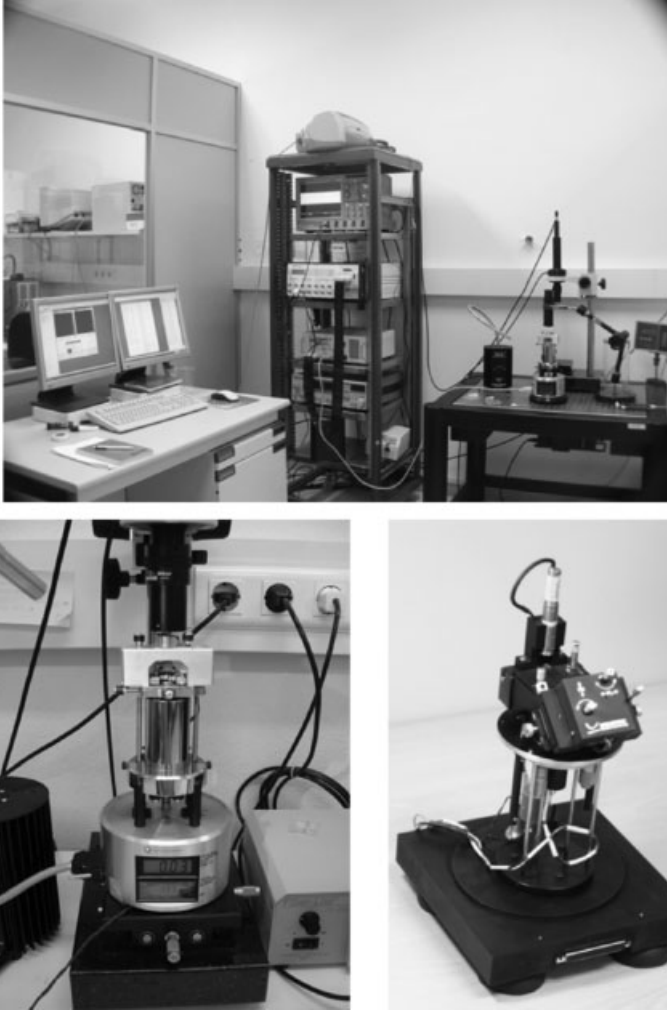
Figure 2.2 Top: microscope setup in 2006. Bottom: images of two commercial microscope bases. The microscope base integrates the detection, the cantilever tip, and the tip sample units.
